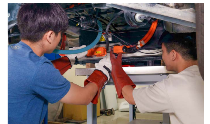
Students conducting battery diagnostics in the EV Lab.
